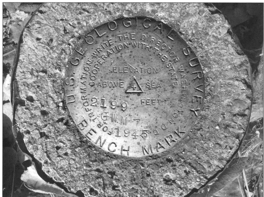
This USGS benchmark, set in 1945, notes the elevation of Chee Chee Flat at 2199 feet.
