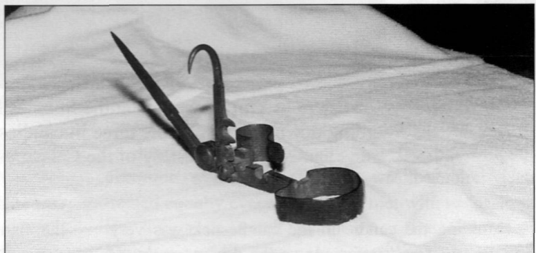
Fancy Model - This fancy model of a candlestick has several accessories. It is a folding model with a hinge in the spike, and it has a blasting fuse cutter and cap crimper. This elaborate model was "invented" by Dave Baratini and donated by him to the Old Timer's Museum in Murphys.
