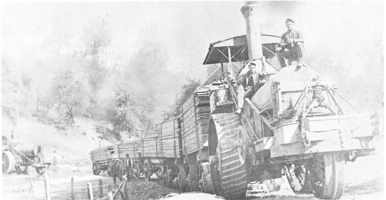
Raggio Bros. steam tractor helped revolutionize Calaveras County lumber industry after turn of century.
