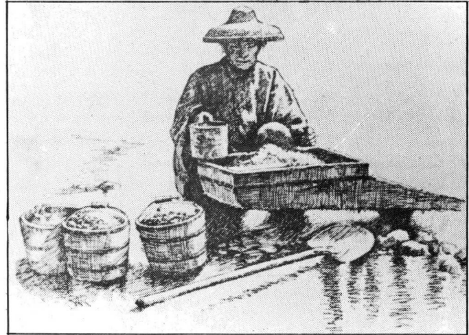
Placer mining with rocker.
